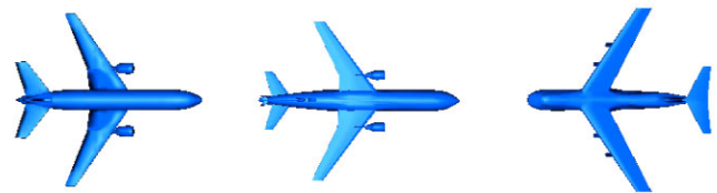
Fig. 2 Three airplane models after PCA-based pose normalization: major axes are correctly found but the front of the fuselage of the right-most model is in the opposite direction
